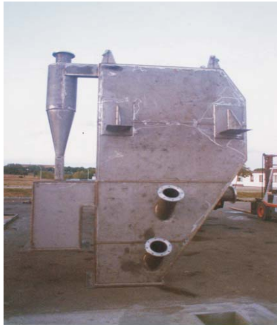
Photo - 3: Gasifier and cyclone assembly
