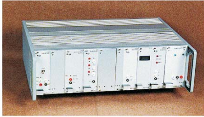
Figure - 3: Reactor Power Monitoring Channels
